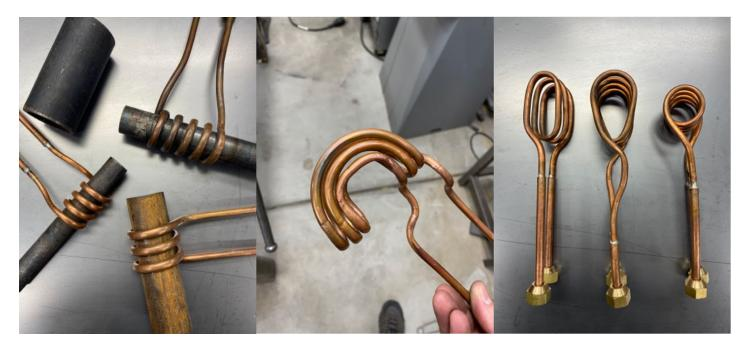
In this workshop we will demonstrate techniques for making a variety of coils, and coach you on making jigs, custom tools, and additional coils for your induction heater.
